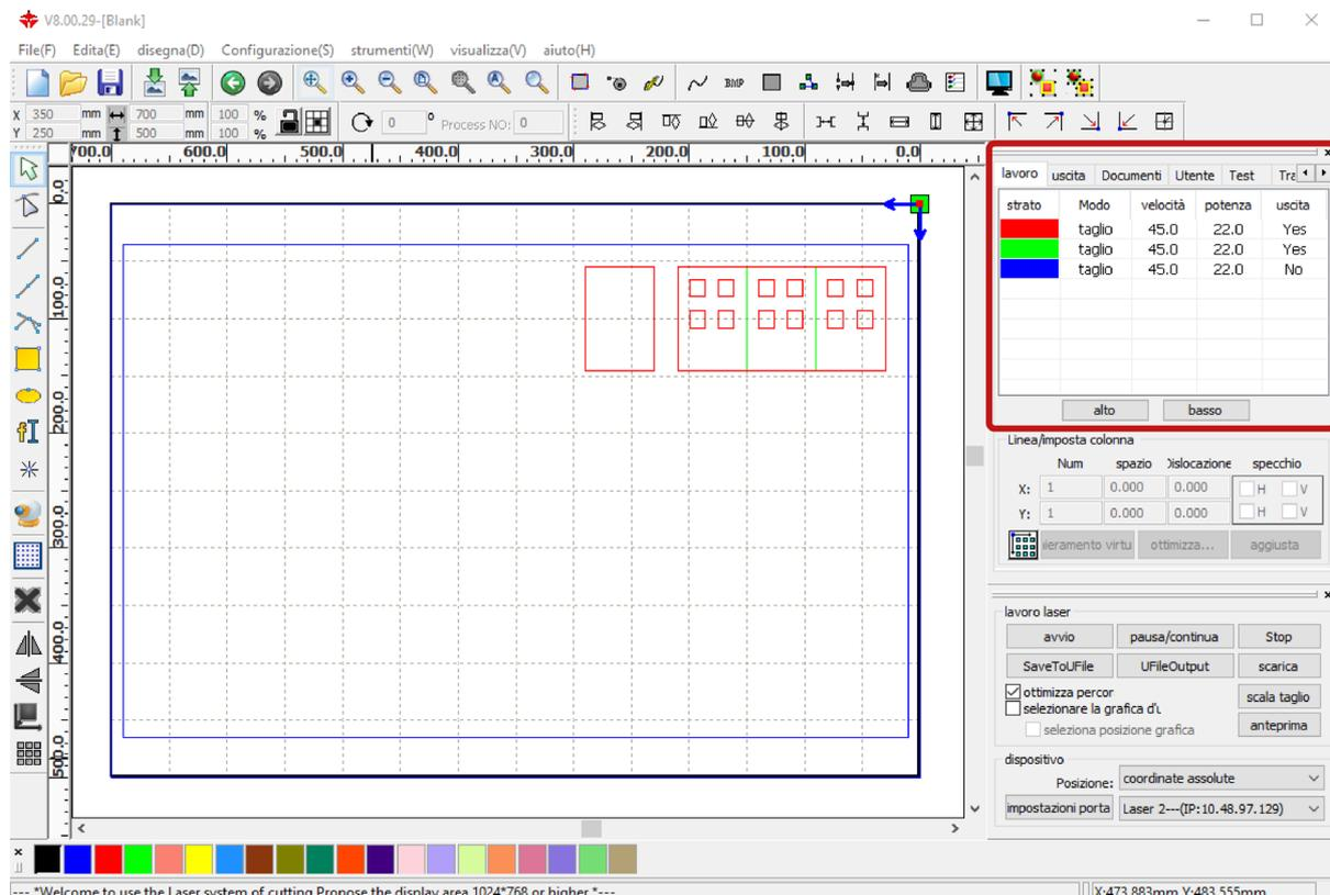
In the top right panel in the section *lavoro*, double-click on one of the layers to open the related window *livello parametri*.
