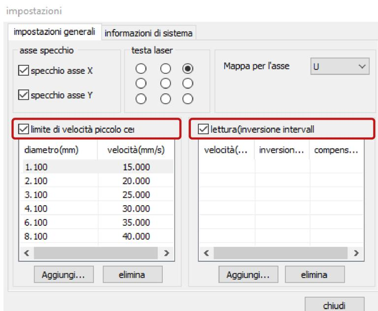
Then in the latter section **click the button *Aggiungi*** (add) and enter the following values of ***velocità*** (speed) and ***inversione*** (inversion) of the **plotter connected** to the pc you are using.
