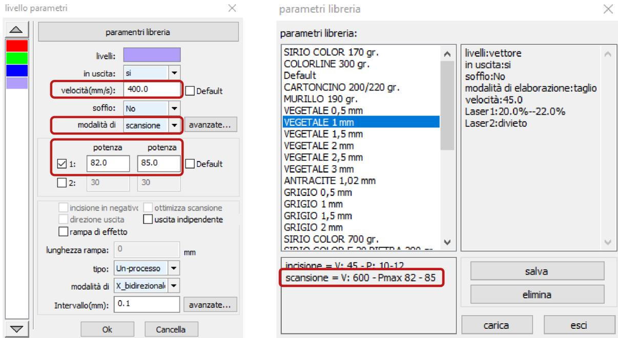
In the **window livello parametri**, in addition to speed and power parameters, it is necessary to check the **parameter soffio** (blow), which is advisable to set to **No** in the case of procedures in **modalità di scansione** to keep the surface of the material cleaner.
