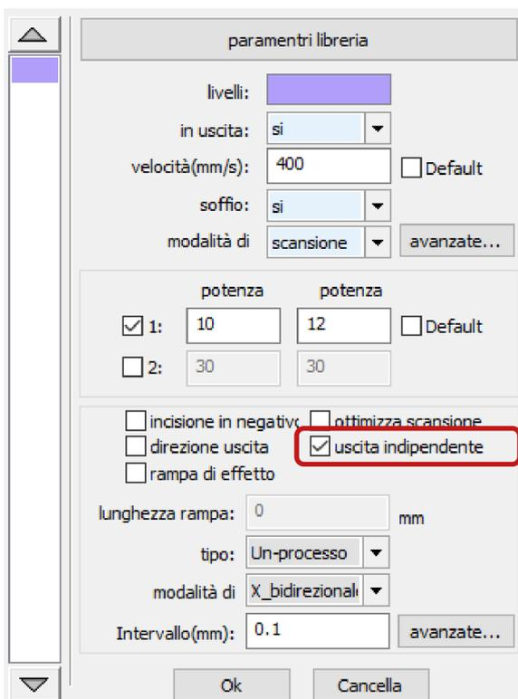
In the **top-right panel** in the section **lavoro**, **double-click on the layer** that contains the scans to open the related window **livello parametri** and activate the item **uscita indipendente** (independent output).
