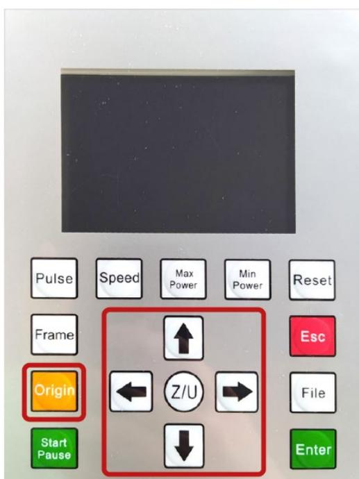
On the **control panel** of the machine, **move the laser head with the arrows** until you reach the desired point for the **start of the cut**, then press the **Origin** button to record it as **posizione corrente** (current position). This relative origin **remains valid** for all the following cuts that are set in **posizione corrente**, until the input of a **new Origin** or until the plotter is turned off.
