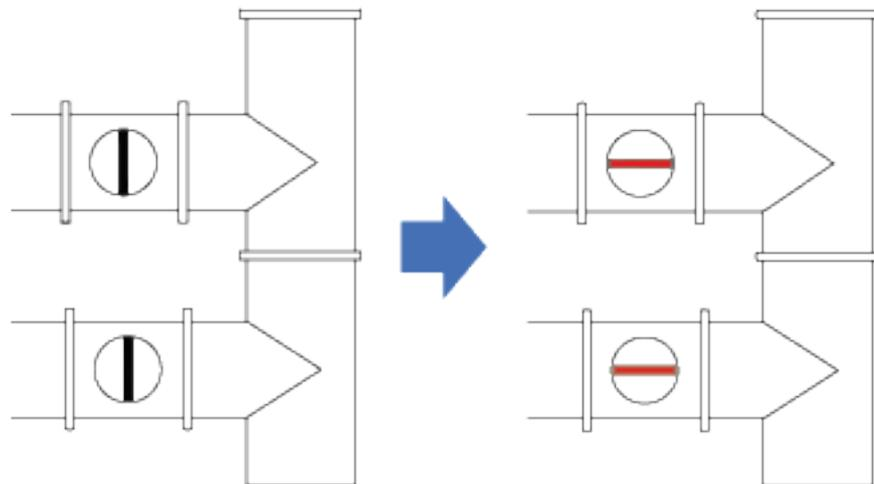
In the case of laser plotters, **the air system** not only eliminates cutting fumes, but also **helps to keep the material still and adherent to the honeycomb panel**, preventing the laser beam from going out of focus and the cut pieces from moving. Therefore, to ensure the **best possible aspiration**, check that the **dampers** on the pipes connected to **machines** that are **not in use are closed**, including the *hot wire cutter*.
