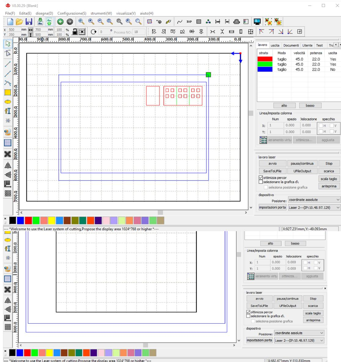
In this case too, it will be necessary to **edit the file** and place the pieces inside a 1000 x 700 mm frame **or** (if available) **use lasers 1 and 2** to cut the pieces.
