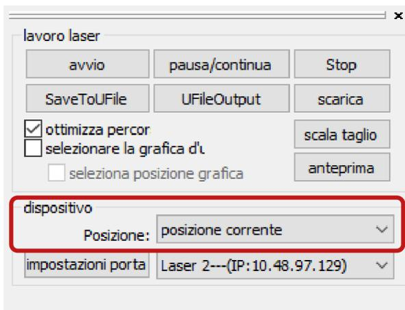
In order to determine the current position, the software considers all drawn elements, even if they are placed on layers that will not be cut, such as **frames**, which is why **they must be deleted directly in RDWorks**.
