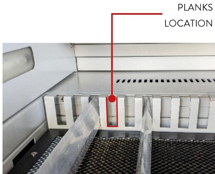
**TURN OFF THE PLOTTER**, by turning the **key on the right side only**, before **taking the planks** which are located inside the machine. **Open the front door** with the specific key that is found in the drawer CS1 of the CNC lab, **pull out the planks**, then **close the panel** and **restart the plotter**.
