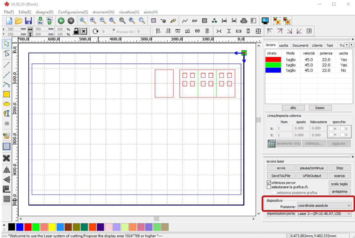
For some cuts, however, it may be useful to set a **starting point of the cut** relatively to the drawn geometries, by setting in the panel **lavoro laser**, on the bottom right, the item **Posizione:** in **posizione corrente** (current position).
