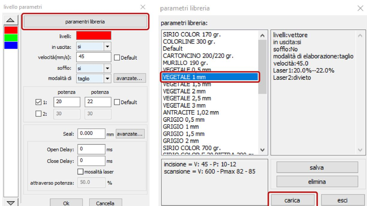
This choice only concerns the assignment to a layer of the **cutting** parameters of a **given material** of a **given thickness**.
