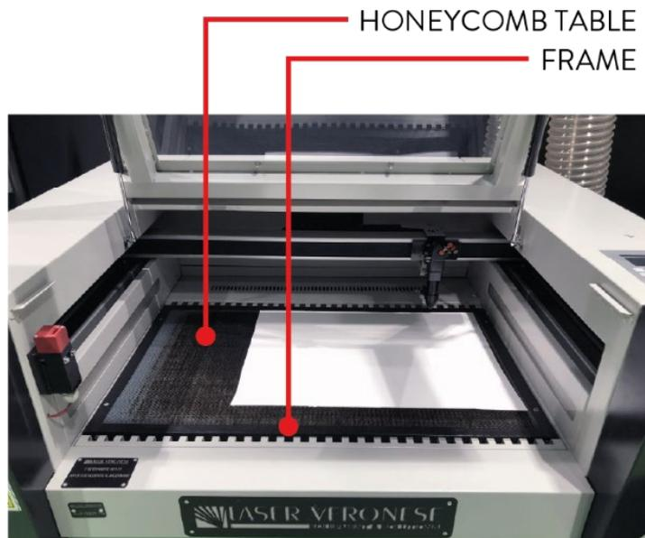
To cut **rigid sheets**, such as **methacrylate**, and achieve the best cutting cleanliness, it is necessary to **place the material on bars** and not on the honeycomb panel.
