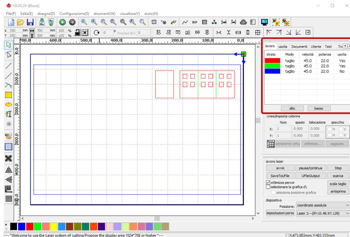
In the top right panel, in the *lavoro* (work) section, the layers created by the software are presented with the **processing parameters**: *Modo* (method), *velocità* (speed), *potenza* (power) e *uscita* (output), that were set for that colour in the last working session.
