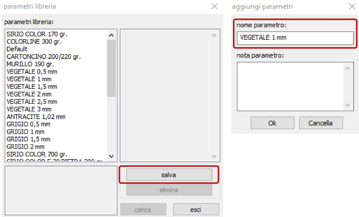
If the ***nome parametro*** that you want to assign **already exists**, it is possible to **overwrite** its parameters to update the material. In this case it is necessary to fill in the item ***nota parametro*** with the values for ***incisione*** and ***scansione*** already determined for that material or with new parameters considered more fitting.
