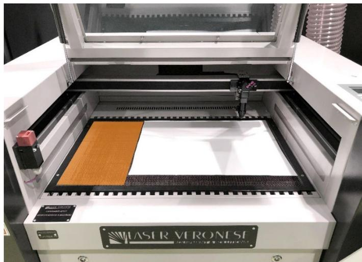
If the **material** to be cut is **smaller than the honeycomb surface** and the aspiration is insufficient to hold it in place, **cover the remaining part of the top with other cardboard**.
