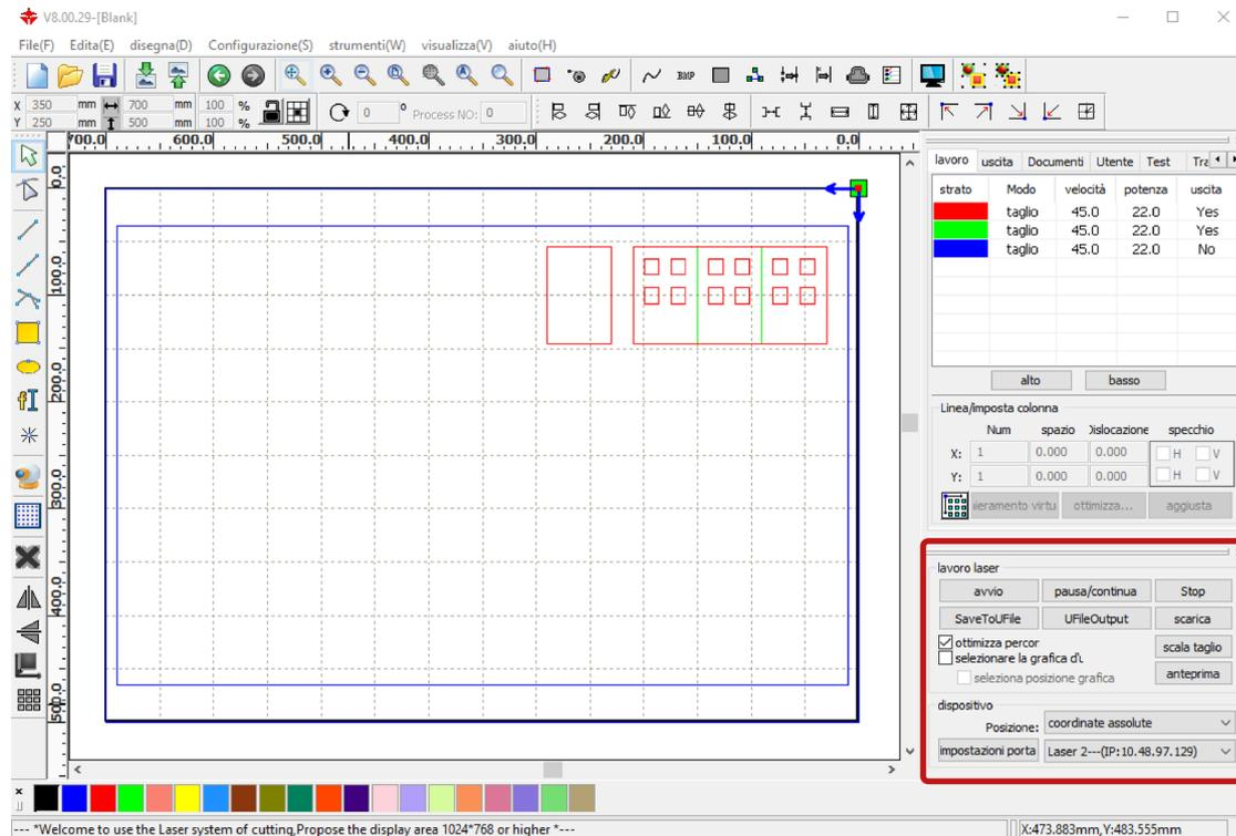
In this panel, before starting the cut, you must define the **starting point** by setting the item *Posizione* (position) in *coordinate assolute* (absolute coordinates) in the section *dispositivo* (device).
