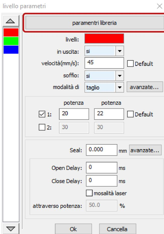
As explained in chapter 4, the parameters for **speed** and **power** to cut and engrave materials are indicated in the **window *parametri libreria***. After the tests for cutting and engraving it may be necessary to **change the parameters** of a material or **add** a new one by saving the settings in the **window *livello parametri***.
