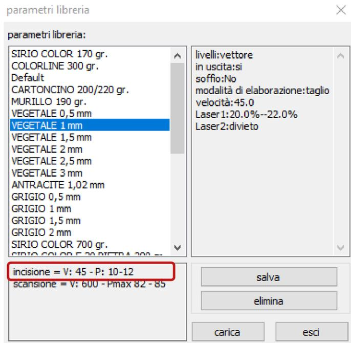
In the window *parametri libreria*, in addition to the parameters of speed and power, you need to check the parameter *soffio* (blow), which in the case of materials such as: **cardboards and similar**, must be set to *si*. While in the case of **methacrylate**, it must be set *No*.
