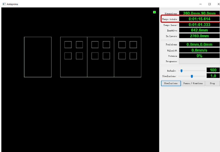
The *Tempo totale* to take into account for scheduling appointments is displayed in the top right panel. By starting the *Simulazione* it will be possible to visualize the path of the cutting head.
