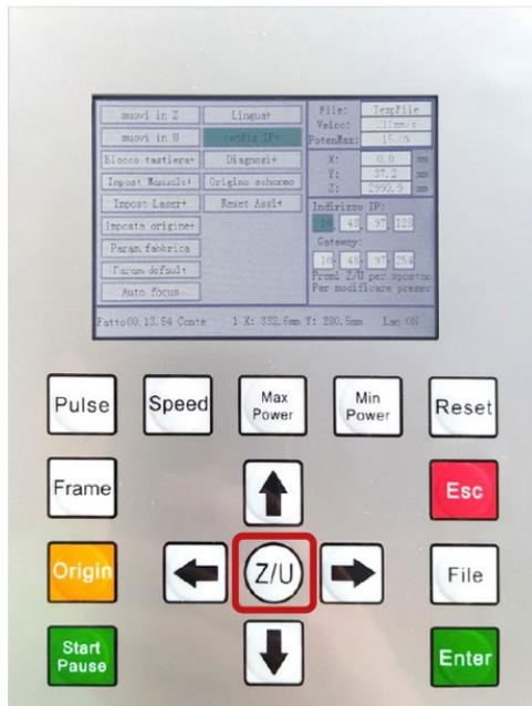
To **read** the IP address of each plotter press **Z/U** > **Config IP+** > **Enter** on the machine control panel. To return to the main menu use the **Esc** button.
