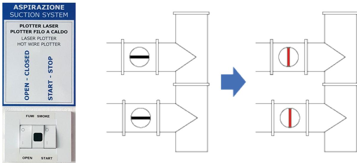
TURNING OFF THE AIR SYSTEM: return in position **O** the two switches on the right of the CNC LAB door.
